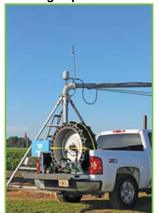
Valley Irrigation's new Revolution airless tire for center pivot systems was on display at Field Day. It includes a non-directional tread that won't plow up fields as it rolls through.
