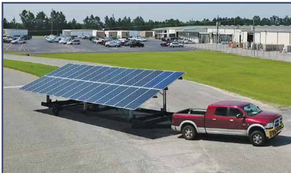
A heavy-duty pick-up truck tows a mobile solar array for installation.
