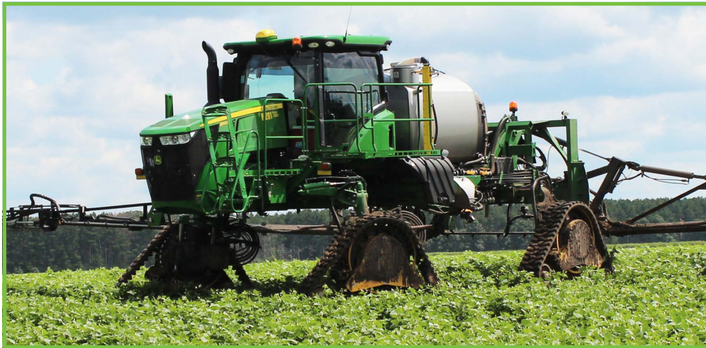
A John Deere sprayer retrofitted with Mattracks rubber tracks that allow heavy machinery to operate in mud, snow and rocky areas without bogging down or significantly compacting the ground. (Provided photo)
