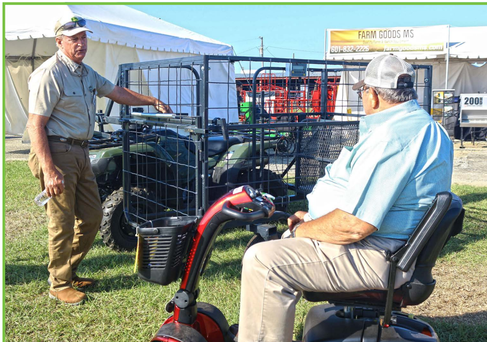
Jim Anderson, a large animal veterinarian and owner of Farm Goods MS based in Carthage, Miss., demonstrates a calf-catcher to a disabled farmer at Sunbelt Ag Expo in October 2018. The calf catcher attaches to most ATVs and UTVs and allows a single operator to safely capture, process and move newborn calves.
