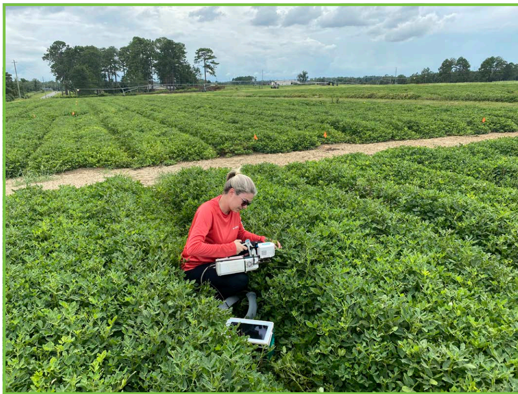
UGA Plant Pathologist Dr. Cristiane Pilon uses an infrared gas analyzer to measure photosynthesis of a peanut plant in a test plot at the University of Georgia Tifton Campus. The peanut plant leaf is placed under the analyzer’s scanner to measure the plant’s efficiency using carbon dioxide to produce energy and release oxygen. (Cristiane Pilon/UGA Tifton Campus)
