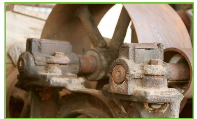
A close shot focuses on a cotton oil wick in that may well be original to this gin. Prior to advancements in the use of ball bearings, the power shafts had wick oilers to prevent them from wearing against the frame.
