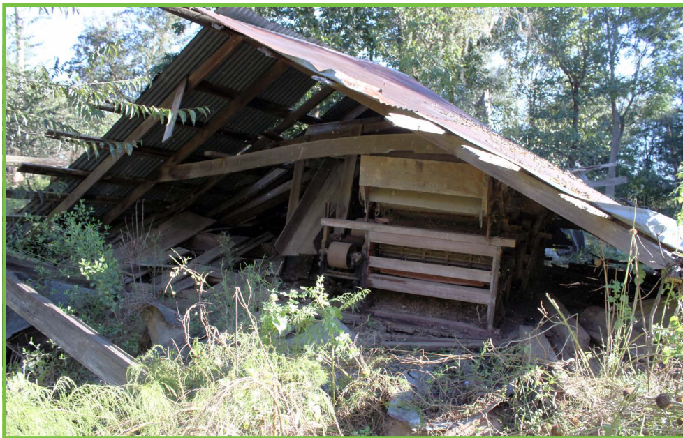
Installed on the second floor of a gin house in the early 20th century, two Lummus gins survived the collapse of the house to be rescued from ruin in October. They are 60-saw models, meaning the wooden cabinets contain 60 saw blades that rotate between flat metal plates to separate cotton lint from the seeds. The lint was removed from the saws’ teeth by horsehair brushes.
