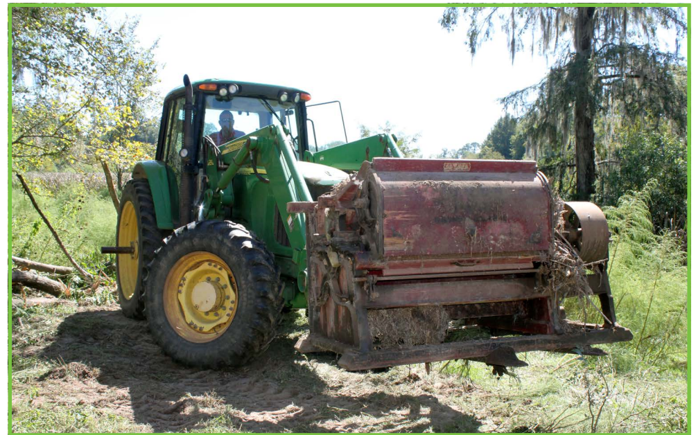
Installed on the second floor of a gin house in the early 20th century, two Lummus gins survived the collapse of the house to be rescued from ruin in October. They are 60-saw models, meaning the wooden cabinets contain 60 saw blades that rotate between flat metal plates to separate cotton lint from the seeds. The lint was removed from the saws’ teeth by horsehair brushes.
