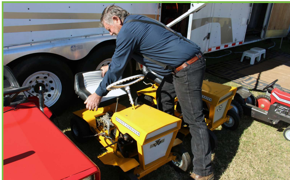
Larry Coomer removes the seat of one of his Massey Ferguson garden tractors to show the transmission, which is almost as big as the engine. The yellow Massey Ferguson garden tractors are part of the Executive series from the early and mid-1960s. The red and grey models came later and were designed to look like the large farm tractors. (Jay Jones/GDA)
