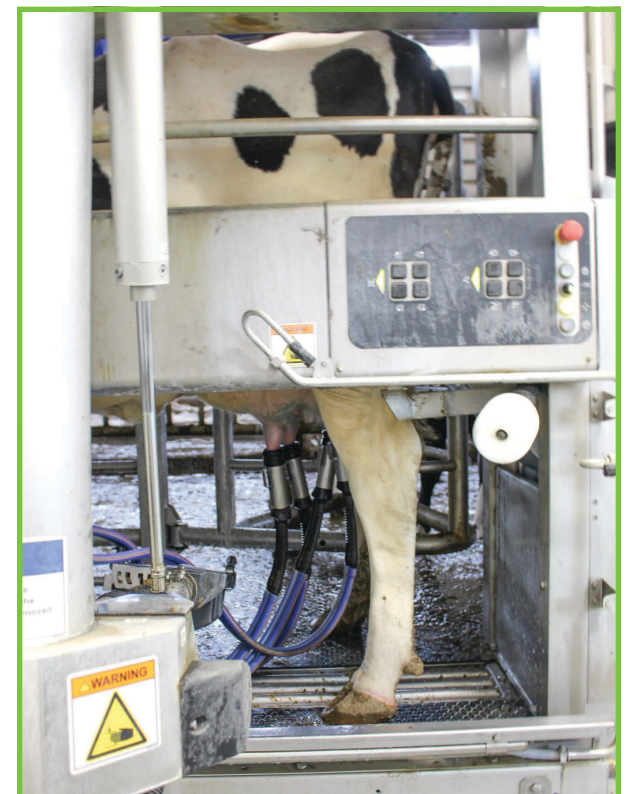
Cows volunteer to get milked on their own with robotic milking systems. Here, a robotic arm cleans the udders and another arm places cups on each teat to begin milking. (Jay Jones/GDA)
