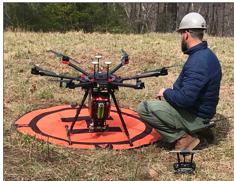
A U.S. Forest Service ranger checks the drone, or unmanned aerial vehicle, before flight during a prescribed burn earlier this year in the Chattahoochee National Forest. The forest service is training rangers to fly the drones and use them in setting and monitoring prescribed burns. (USFS photo)
