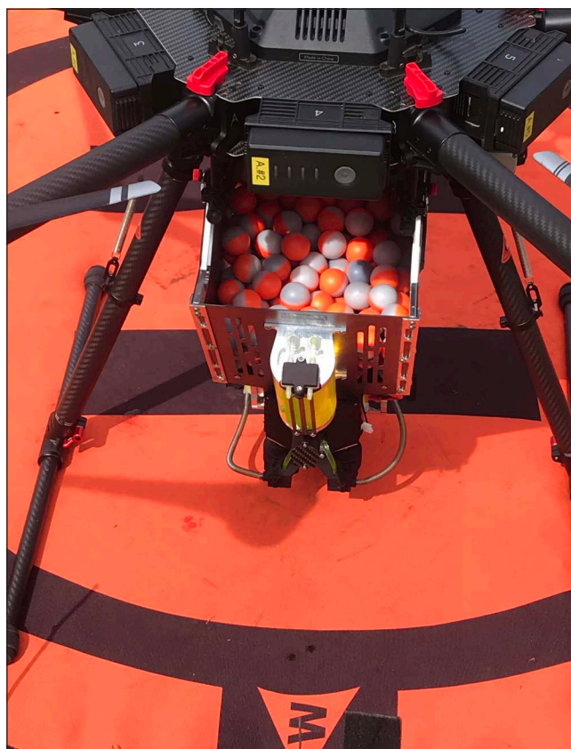
The drone used by the U.S. Forest Service in their training program can set prescribed fires by dropping incendiary spheres in patterns in the area to be burned. Forest rangers and fire professionals can then monitor the fire’s progress with cameras mounted on the drone. (USFS photo)
