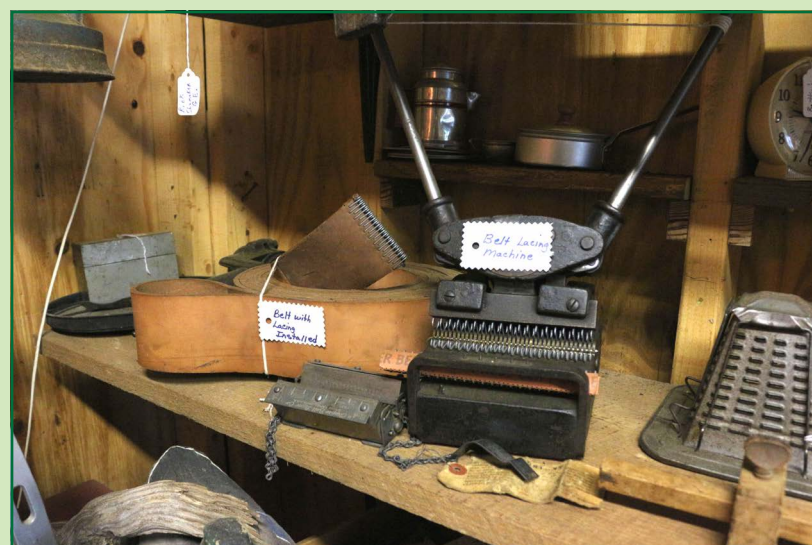
At right, a belt lacing machine allowed farmers to repair broken flat belts used to transfer power from tractors to implements like feed mills and hay balers.
