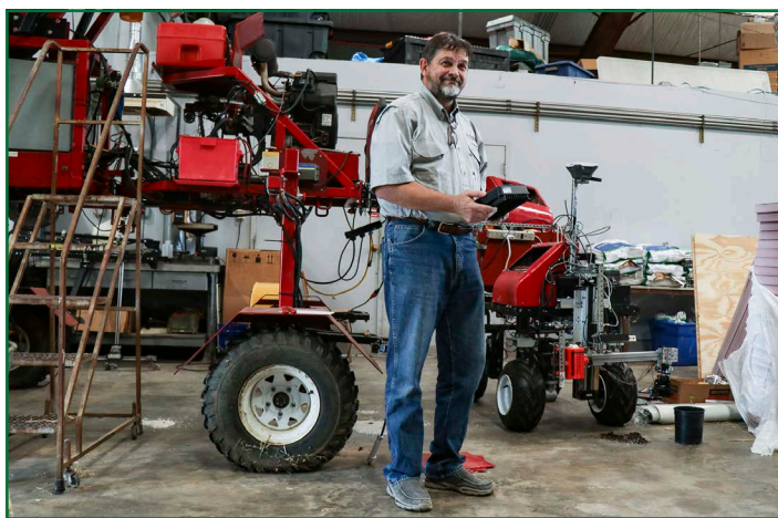
University of Georgia CAES professor Glen Rains holds the control panel to the “Little Red Rover.” The rover is a multipurpose robotic tool that can be used for planting, weed and pest management, and more. (UGA-CAES/Katie Walker)
