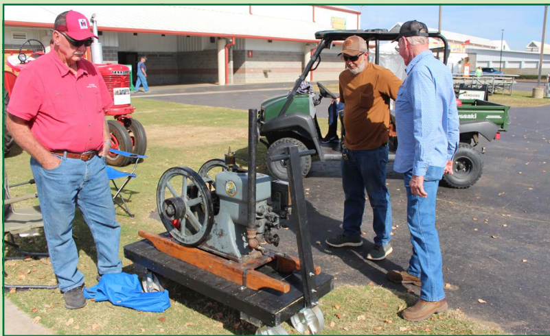
Wayne Dennard, left, and Mel Powell of the Ocmulgee Antique Tractor Club discuss Dennard's 1.5HP Hercules hit-and-miss engine. The engine was built in 1925 and was used to power anything requiring slow, steady belt-driven power, from washing machines to corn grinders. (GDA/Jay Jones)
